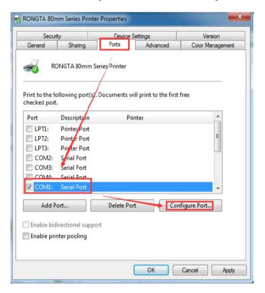
Select the corresponding serial port (take COM1 as an example), select COM1, and then select the configuration port. The following dialog box appears: Set the value of bits per second to be the same as the printer baud rate. If the baud rate is 19200, then set the value of bits per second in the serial port properties selected for printing as 19200.
