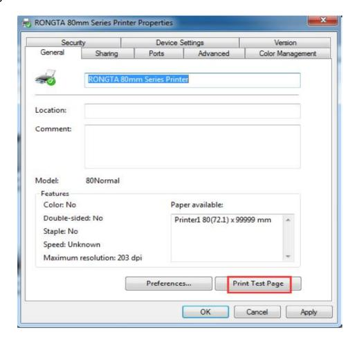
Select "Print Test Page (T)". If the test page can be successfully printed, it means the printer has been connected to the PC and configured correctly, and the printer port can be used normally.
