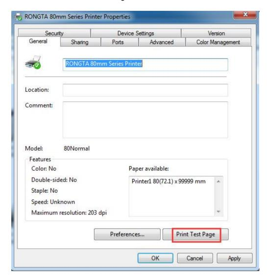
Select "Print Test Page (T)". If the test page can be successfully printed, it means the printer has been connected to the PC and configured correctly, and the printer port can be used normally.
