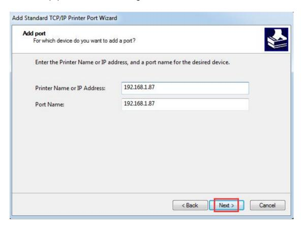
Then enter "192.168.1.87" after the "Printer Name or IP address (A)", and then select "Next (N)", as shown in figure above
