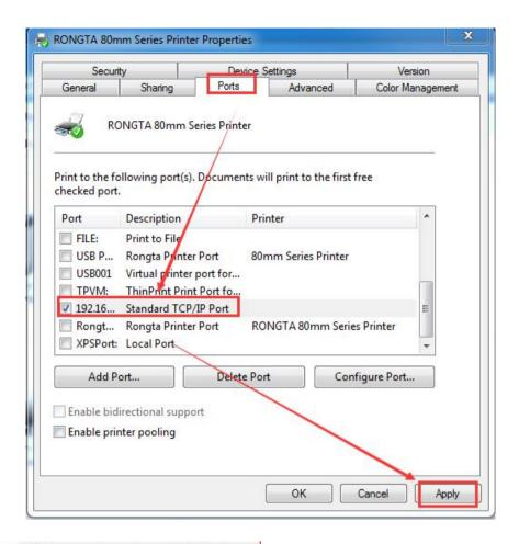
Select "192.16... Standard TCP/IP Port", then select "Apply (A)" as shown in the figure above, select "General" as shown in the figure below.
