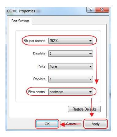
After settings are completed, click "OK" to save the settings. Back to the "Printer Properties" window, select "Apply (A)", as shown in the figure below:
